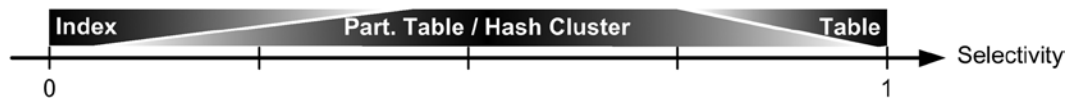
Figure 13-2. Specific access paths work efficiently only for a specific range of selectivity
