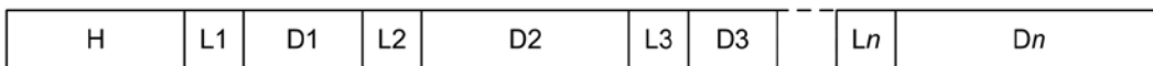
Figure 16-1. Format of a row stored in a database block ( H = row header, L_n = length of column n , D_n = data of column n )
