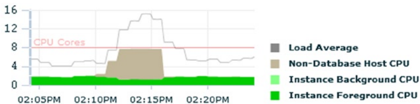
Figure 4-15. The Runnable Processes chart shows the CPU utilization as well as the load average at the database server level.
